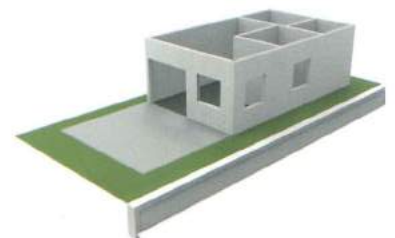
Infill perimeter capping beam
